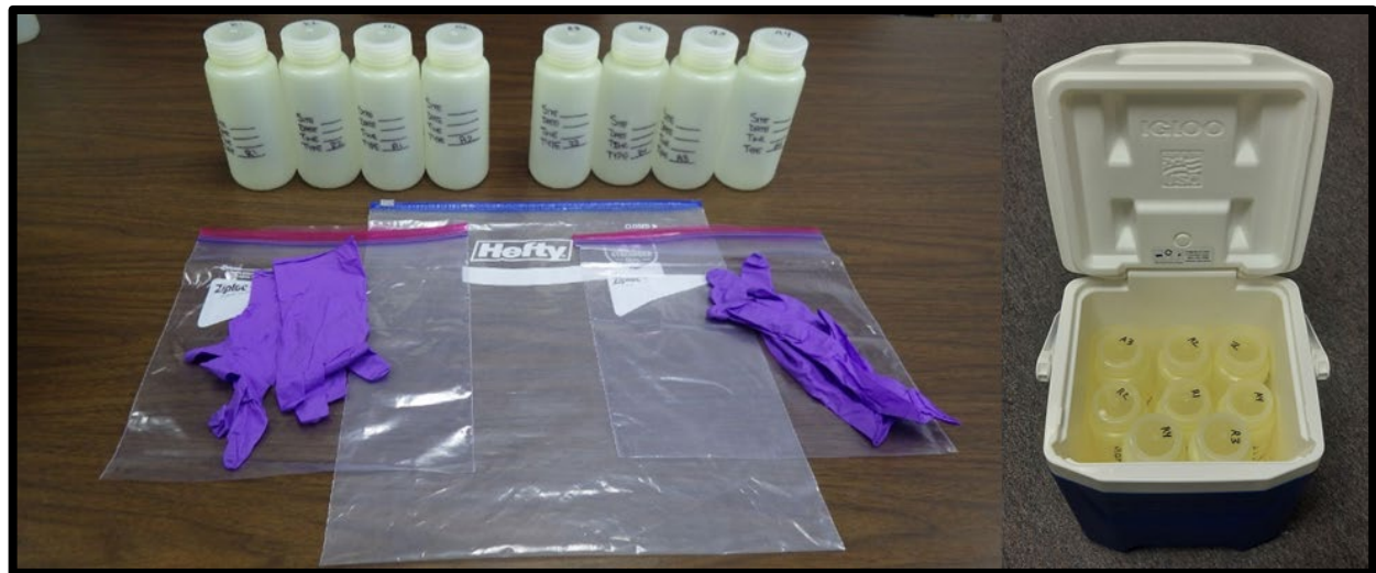
Figure 11 Example of pre-prepared sampling kits used for environmental DNA (eDNA) sampling (left) and self-contained cooler for each sample site (right). All site kits were pre-prepared in a decontaminated, designated space prior to sampling in order to mitigate potential for cross-contamination between sites.
