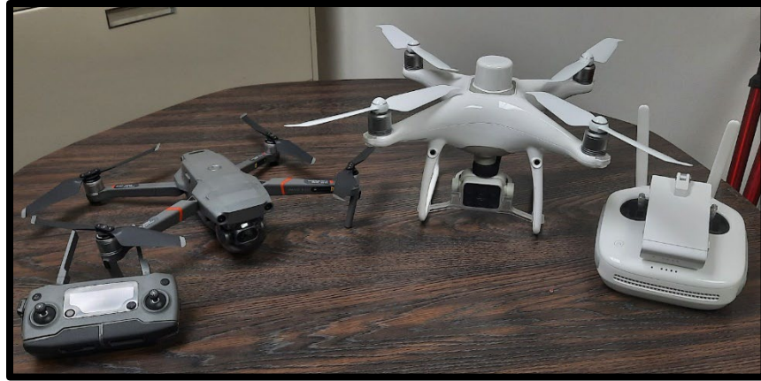
Figure 13 Drone platforms used for aerial surveys: DJI Mavic 2 Dual (Drone M2 ; left) and DJI Phantom 4 Multispectral (Drone P4 ; right).
